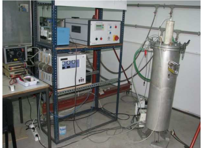
Fig. 15. The experimental setup consisting of the plasma reactor, the DC power supply, the gas generator, vacuum pump and a PC for process control.
