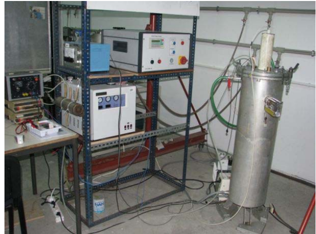
Fig. 15. Experimental setup consisting of the plasma reactor, DC power supply, gas generator, vacuum pump, and a PC for process control.
