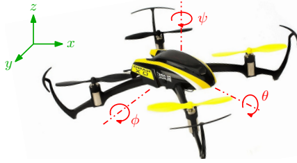
Fig. 11. Representation of the different control variables in the mini quadrotor helicopter.
