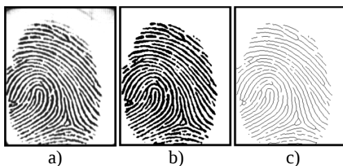
Fig. 5. a) Initial image; b) Segmented and binarized image; c) Thinned image
