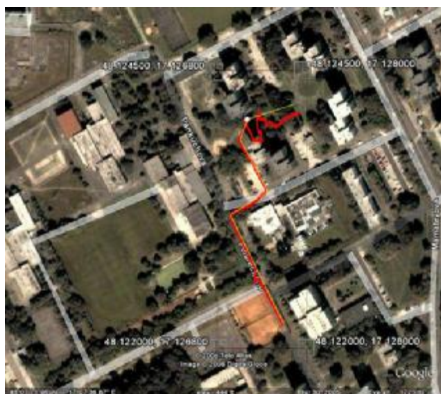
Fig. 5. Comparison of real path (yellow colour) and measured path (red colour) at road with shape of cusped line measurement
