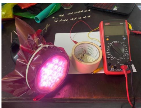
Fig. 4. LDR under the influence of a filtered light stimulus.
