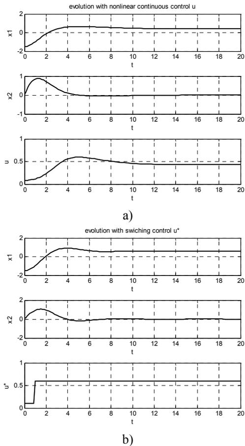
**Fig. 4.** Time-evolution of the position, speed and control signal for the system (19): a) with control (21); b) with switching control (24), (25), (29).
