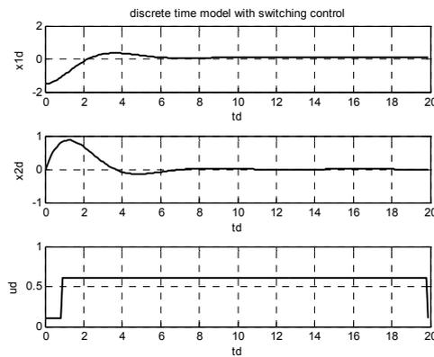
Fig. 10. Time-evolution of the position, speed and control signal for the hybrid system with discrete state equations (35) and (39) and the discrete switching control (40).
