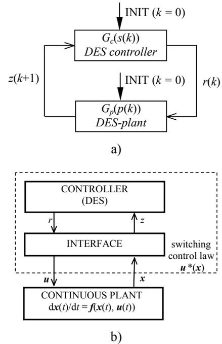
Fig. 2. Modelling approaches of the HCS: a) logical supervision and b) nonlinear control.
