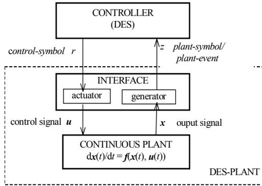
Fig. 1. The architecture of a hybrid control system.
