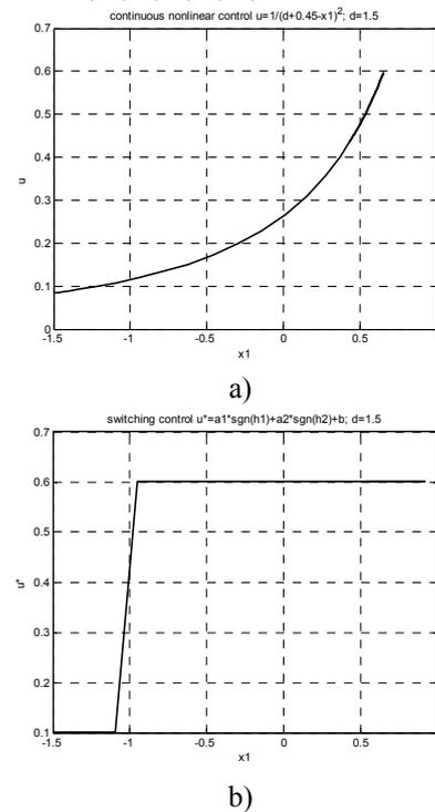
**Fig.5.** Graphical representation of the control-position dependence: a) with the control law (21); b) with switching control (24), (25), (29).
