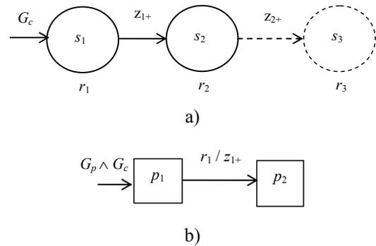
Fig. 8. DES controller and the controlled DES-plant automaton ; in a) the state  $s_3$  is not entered, in the closed loop dynamics, because system reaches an equilibrium in  $p_2$ .
