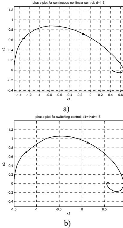
Fig. 6. Phase plot of the system (19) driven by a) the nonlinear control (21) and b) the switching control (24), (25), (29).
