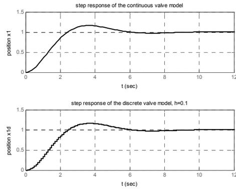
Fig. 9. Step responses of the mass position of the mechatronic system in case of the continuous state equations (19) (up) and of the discrete time model given by (35) and (39).
