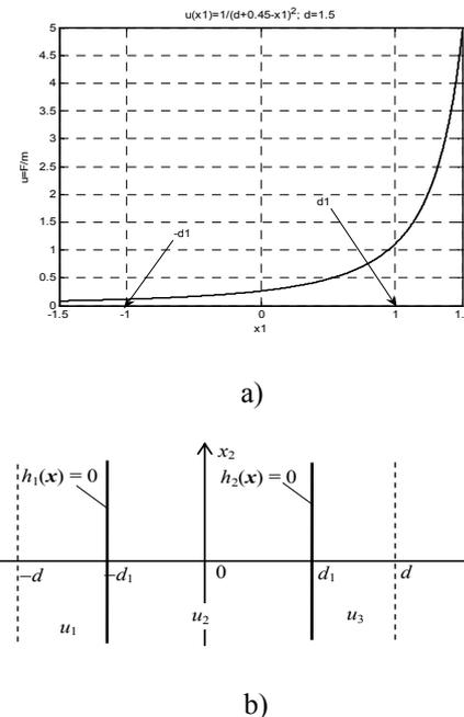
Fig. 3. a) Simulation of the nonlinear control (21) and limits of the partition on the  $x$ -axis; b) the state space partition for the system (19).
