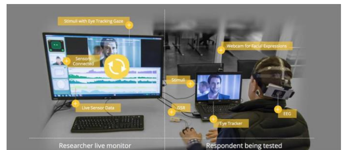
Fig. 1. The standard setup for emotion detection by iMotions and Emotient. Image retrieved from (Emotient, 2020).
