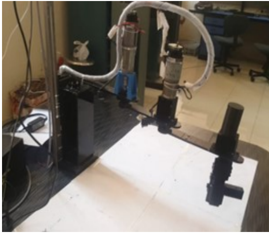
Fig. 11. Hardware setup of 3R planar robot: The encoded Maxon drive system is controlled with myRio-1900 controller to implement the control scheme.
