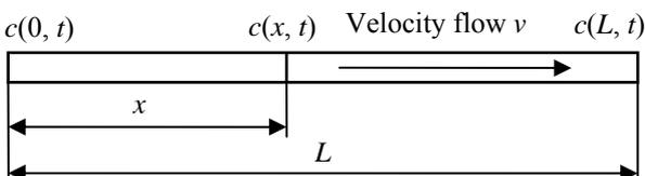
Fig. 1. Chlorine distribution in a pipe
