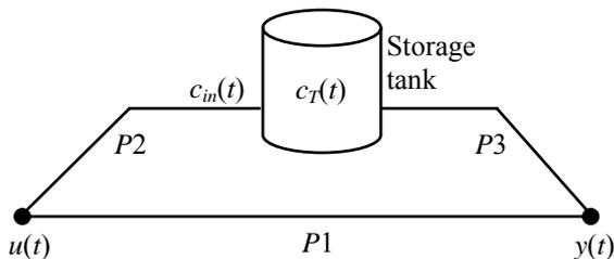
Fig. 5. A simple water network with one tank
