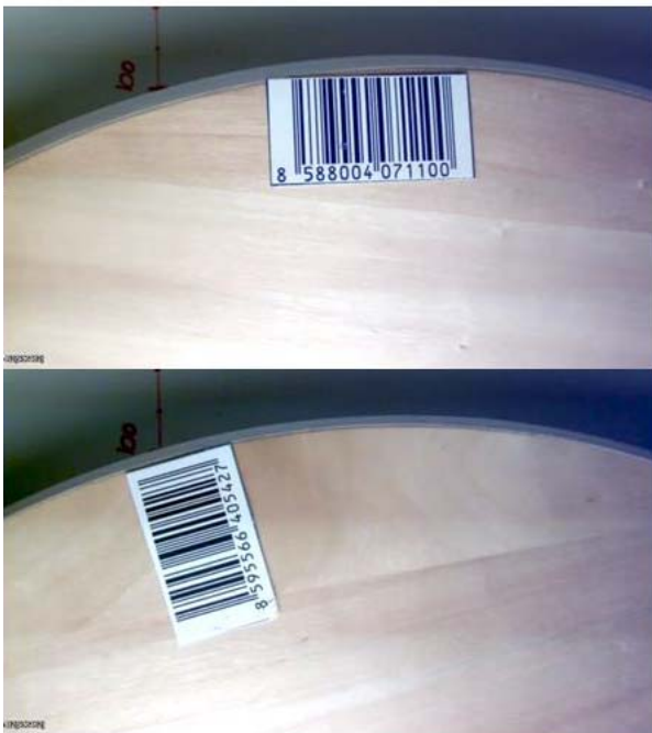
Fig. 12. Rolling shutter effect - static image.
