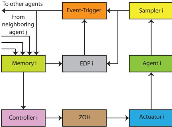
Fig. 1. A distributed event-triggered scheme for MASs
