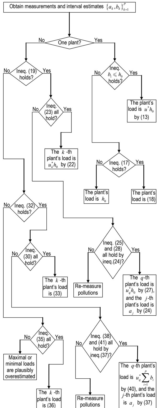
Fig. 1. Algorithm of distributing treatment loads.
