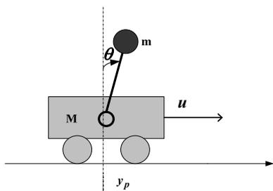
Fig. 1. Schematic of the inverted cart-pendulum.
