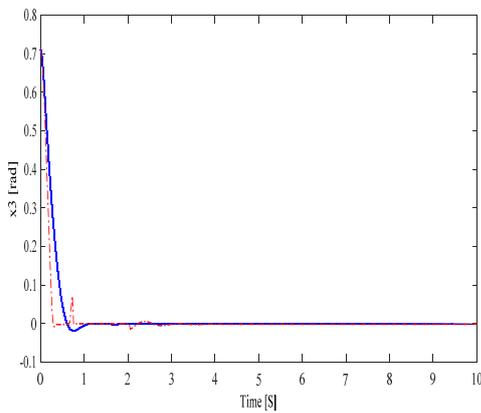
Fig. 4. Evolution of the pendulum angle (dashed line: the proposed approach; continous line: multi-diffeomorphism method).
