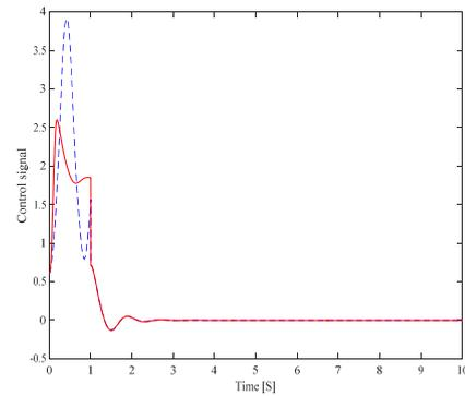
Fig. 5. Evolution of the control signal (dashed line: the proposed approach; continous line: multi-diffeomorphism method).
