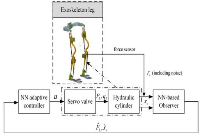
Fig. 3. Diagram of force adaptive NN tracking control scheme with NN observer.
