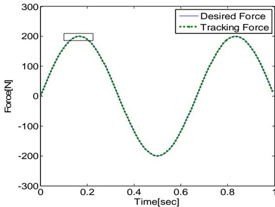
Fig. 9. Tracking trajectories with desired force of  $F_{ld} = 200 \times \sin(3\pi t)$
