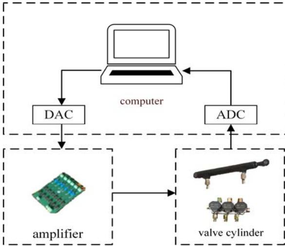
Fig. 8. Block diagram of LEPEX servo system for NN-observer-based force adaptive tracking control.
