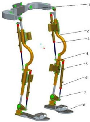
Fig. 1. Structure of the LEPEX 1-Hip 2-Thigh 3-Thigh Drive Cylinder 4-Shank 5-Bound Device 6-Shank Drive Cylinder 7-Ankle 8-Sole.
