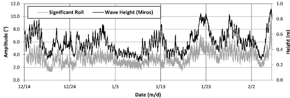
Fig. 12. Evolution of significant wave height measured with a nearby MIROS radar compared with significant roll.
