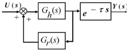
Fig. 3. Thermal HFE scheme with recycle and time-delay.
