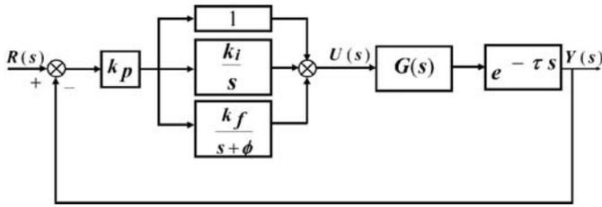
Fig. 1. Proposed control strategy  $PI_f$  in closed-loop with the system (1).
