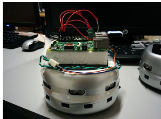
Fig. 4. Modified Khepera III robot with Raspberry Pi 2 B and Wi-Fi dongle.
