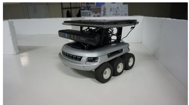
Fig. 5. Koala Rrobot connected via serial to a 13.3" laptop mounted on a support. A Kinect sensor is mounted on the robot and connected directly to the laptop via USB.
