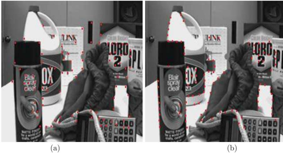
Fig. 4. Features detected (red dots) using “goodness” criteria for texture and edge in (a) and (b) respectively. The results in (a) are from Shi and Tomasi (1994) paper. The adaptation to edge features is shown in (b).
