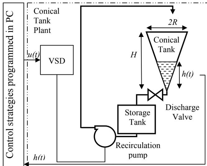
Fig. 2. Control diagram of the conical tank plant.
