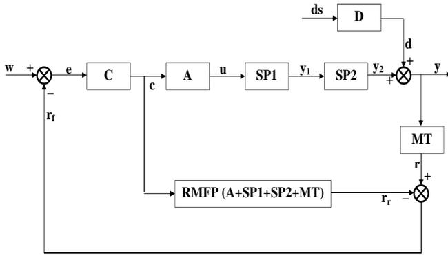
Fig. 8. The control structure based on the IMC strategy.
