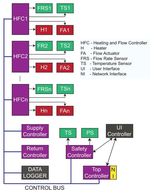
Fig. 4. Cyber part of HIPEC equipment as Cyber-Physical System.
