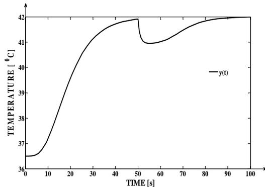
Fig. 13. The control structure response, if the disturbance occurs in the system, for  $H_{C1}(s)$ .
