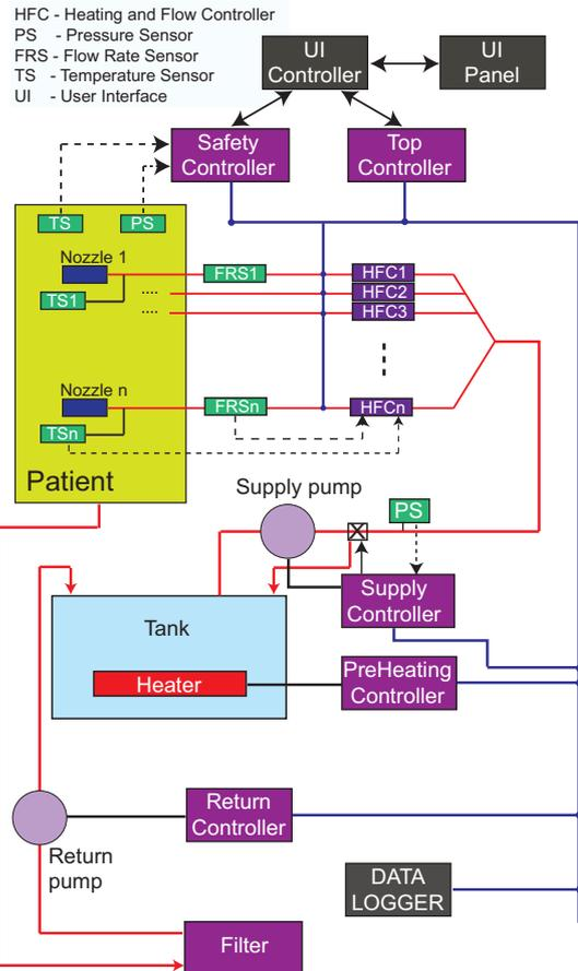
Fig. 3. The essential blocks of the proposed HIPEC equipment architecture.
