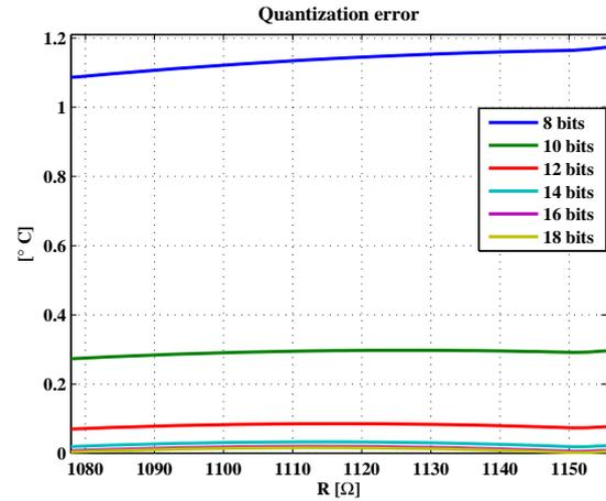
Fig. 6. Quantization error in the proposed wireless system.
