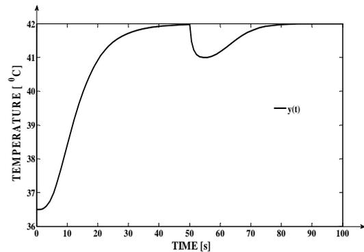
Fig. 11. The control structure response, if the disturbance occurs in the system.
