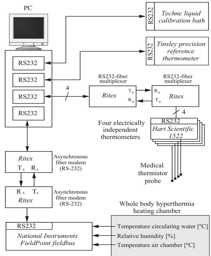
Fig. 7. Example of complex temperature monitoring system (Hjertaker et al., 2005).
