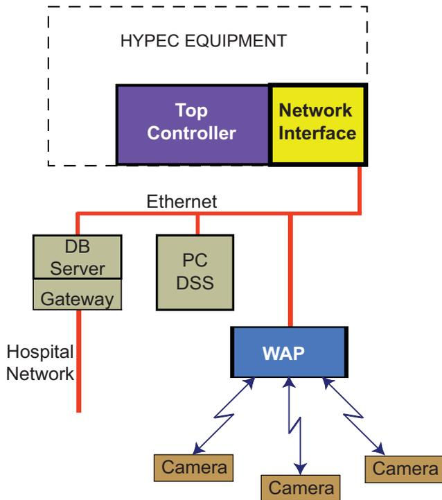
Fig. 2. The integrated HIPEC System.
