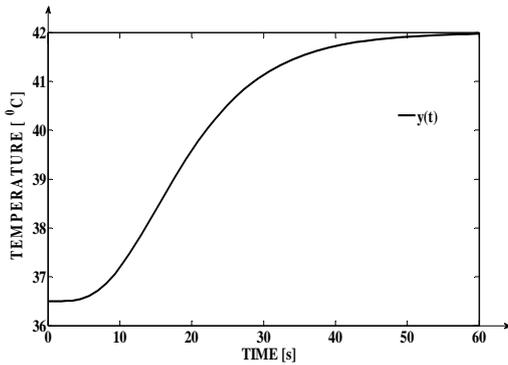
Fig. 12. The control structure response for  $H_{C1}(s)$ .
