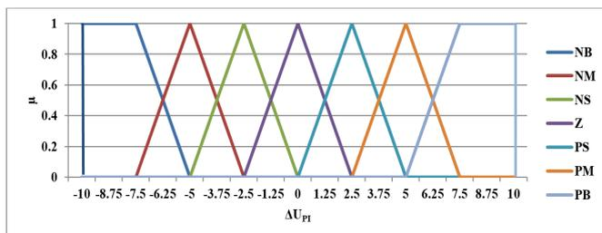
Fig. 7. Output MF for T1 PI FLC
