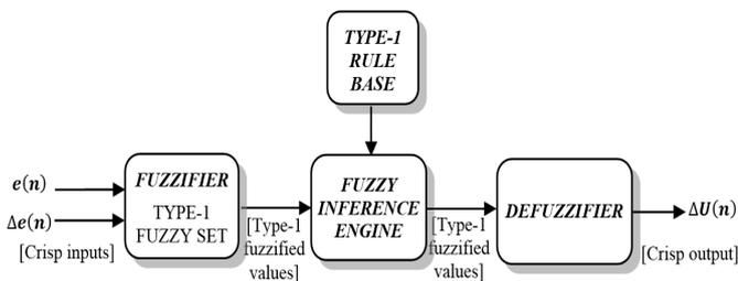
Fig. 5. Structure of T1 PI FLC.
