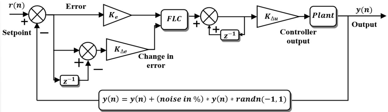
Fig. 1. Block diagram implementation of FLC.
