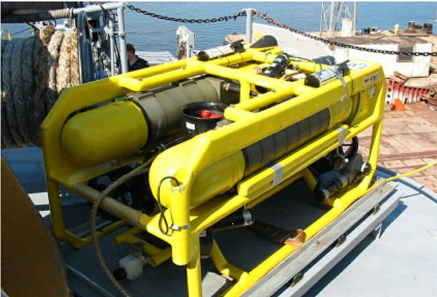
Fig. 6. Underwater vehicle Ukwial designed by Gdansk University of Technology.
