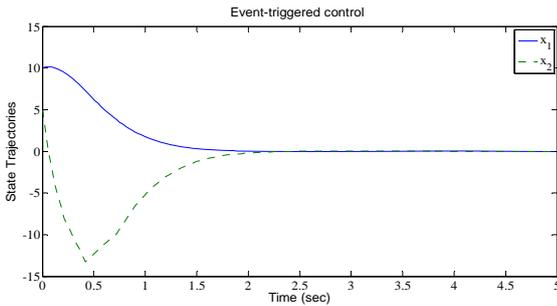
Fig. 5.State evolution under event-triggered control.
