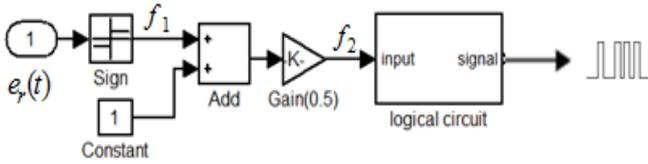
Fig. 2. Event-triggered signal generating circuit.
