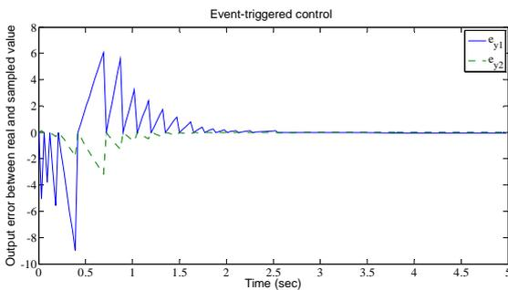
Fig. 7.  $e_y(t)$  under event-triggered control.
