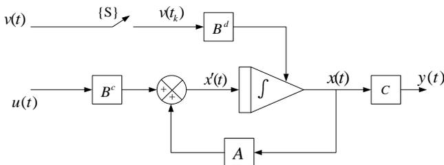
Fig. 1. Structure of PCHS controller.
