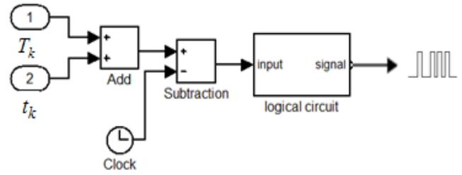
Fig. 3. Self-triggered signal generating circuit.
