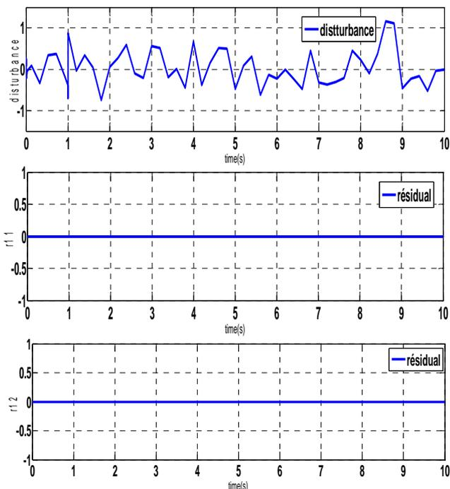
Fig. 5. Insensitivity of residuals to disturbance
