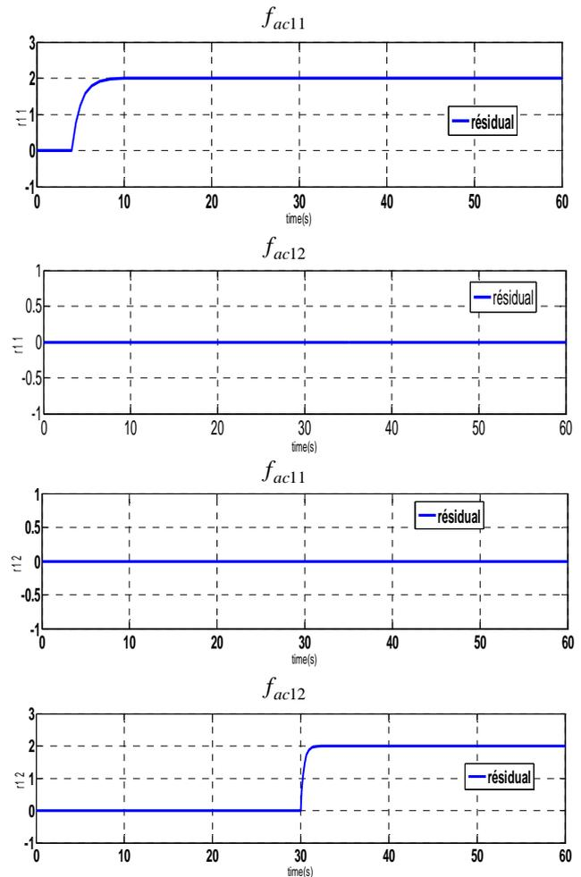
Fig. 6. Table of residuals without measurement noise (UIO1).
