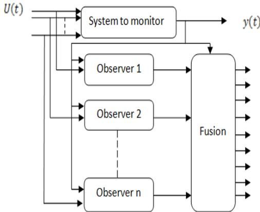
Fig. 1. Bank of observers DOS for actuators faults detection.
