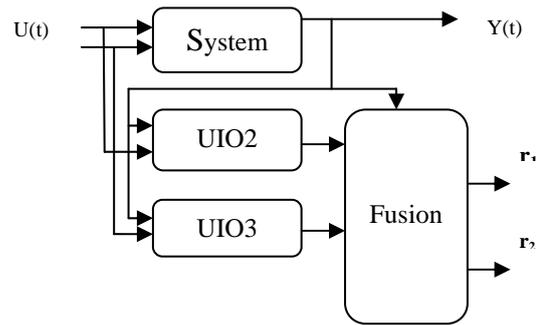
Fig. 4. Bank UIOs (DOS) for the detection of actuators faults
