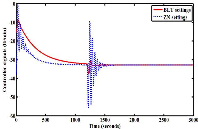
Fig. 15. Manipulated variable (reboiler steam flow rate) for variations in bottom product for increase in feed flow rate at 1200s (Regulatory responses of PI controller tuning using ZN and BLT).
