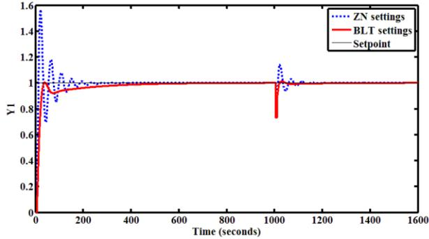
Fig. 17. Controller performance of perturbed system for unit step change  $Y_{1(set)}$  in top product.
