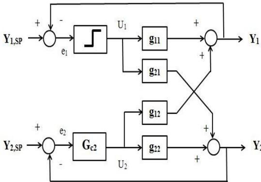
Fig. 3. Step 3 of sequential tuning for 2x2 MIMO system.
