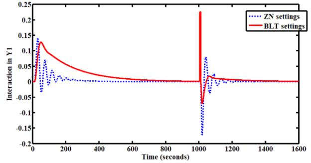
Fig. 20. Controller performance of perturbed system of interaction in  $Y_1$  for unit step change  $Y_{2(set)}$  for top product.
