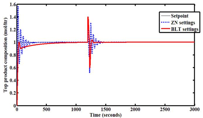
Fig. 12. Variations of top product for increase in feed flow rate at 1200s (Regulatory responses of PI controller tuning using ZN and BLT).
