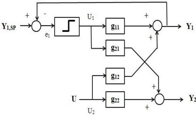
Fig. 1. Step 1 of sequential tuning for 2x2 MIMO system.
