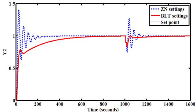
Fig. 19. Controller performance of perturbed system for unit step change  $Y_{2(set)}$  in bottom product.
