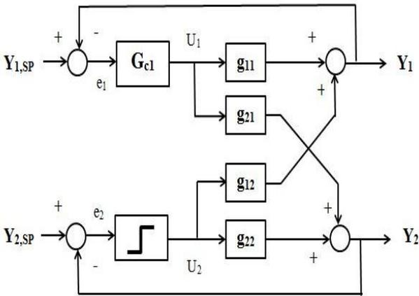
Fig. 2. Step 2 of sequential tuning for 2x2 MIMO system.
