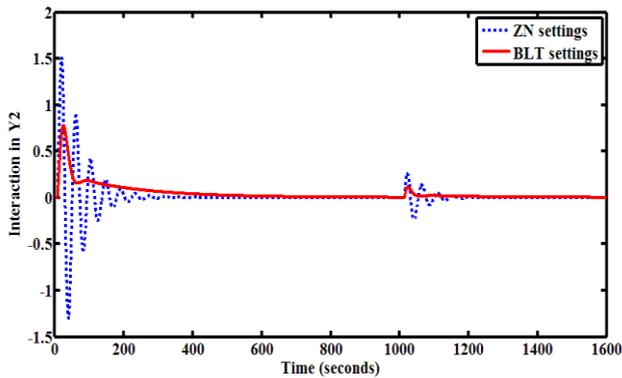
Fig. 18. Controller performance of perturbed system of interaction in  $Y_2$  for unit step change  $Y_{1(set)}$  for bottom product.
