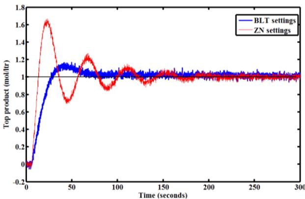
Fig. 23. Variation of top product with measurement noise for unit step change.
