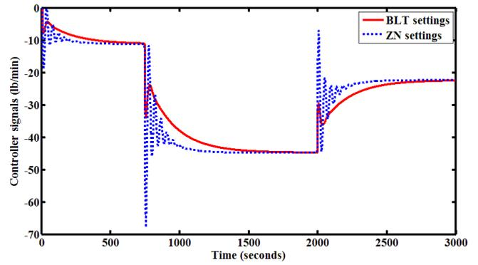
Fig. 11. Manipulated variable (reboiler steam flow rate) for variation in bottom product for multiple setpoint tracking.
