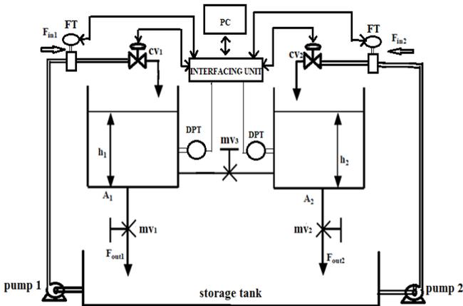
Fig. 25. Schematic diagram of two tank interacting system.
