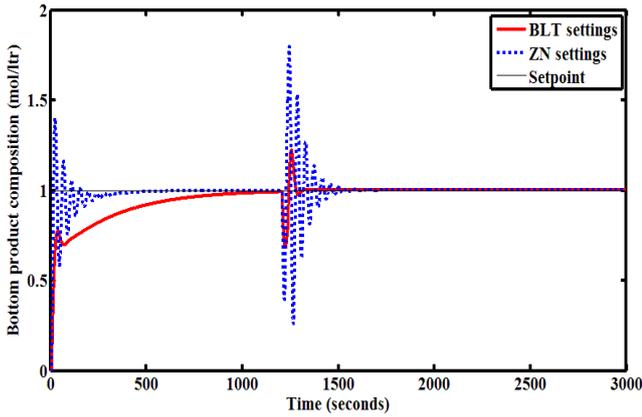
Fig. 14. Variations of bottom product for increase in feed flow rate at 1200s (Regulatory responses of PI controller tuning using ZN and BLT).
