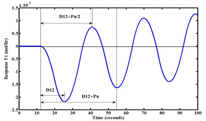
Fig. 5. Relay response for  $G_{p12}$ .
