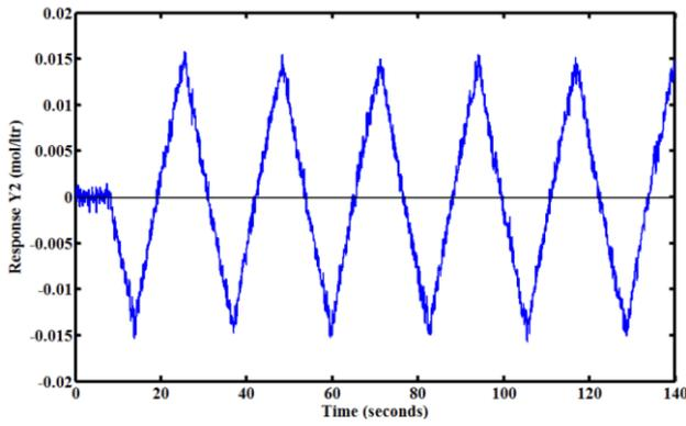
Fig. 22. Relay response for  $G_{p21}$  with measurement noise.
