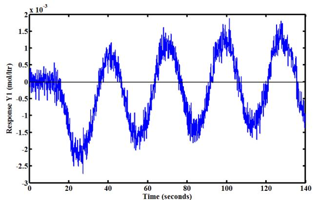
Fig. 21. Relay response for  $G_{p12}$  with measurement noise.
