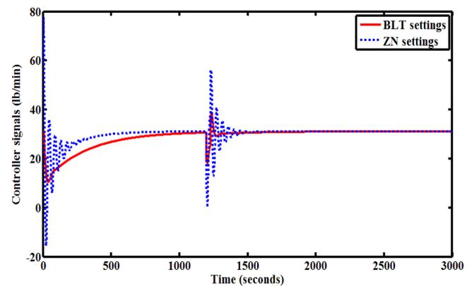
Fig. 13. Manipulated variable (reflux steam flow rate) for variations in top product for increase in feed flow rate at 1200 s (Regulatory responses of PI controller tuning using ZN and BLT).
