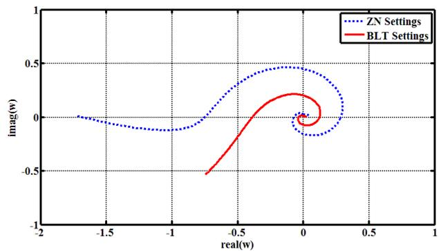
Fig. 16. Stability Analysis of MIMO system using Nyquist Plot.
