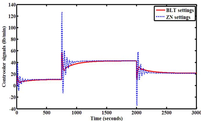
Fig. 9. Manipulated variable (reflux steam flow rate) for variation in top product for multiple setpoint tracking.
