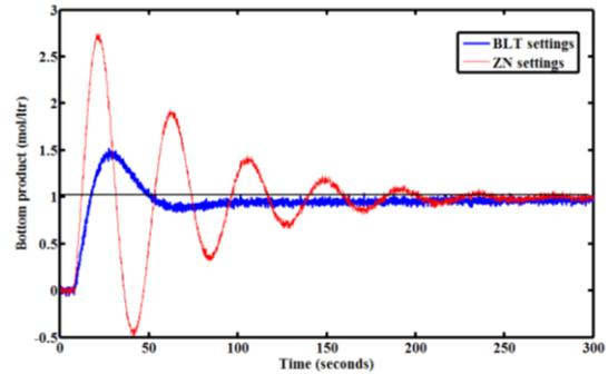
Fig. 24. Variation of bottom product with measurement noise for unit step change.
