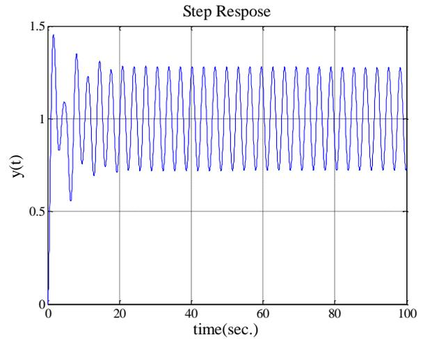
Fig. 4. Step response of the system for the values  $k_p = 0.06778$ ,  $k_i = 3.952$  and  $k_d = 0$ .
