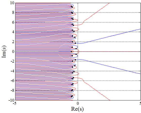
Fig. 10. The roots of the characteristic polynomial for  $k_p = 10.1034$ ,  $k_i = 12.96$  and  $k_d = 0.3$ .
