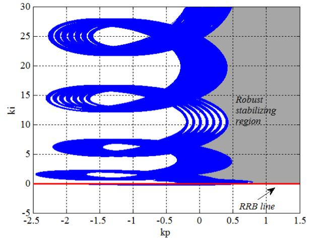
Fig. 11. Robust stability region for a PI controller in the  $(k_p, k_i)$  parameter space.
