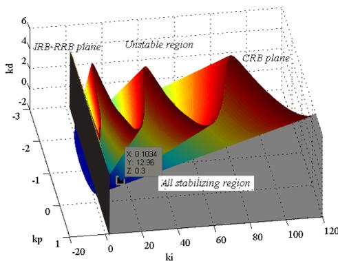
Fig. 6. Stability region for the *PID* controller parameters in the  $(k_p, k_i, k_d)$  parameter space.
