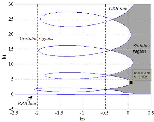
Fig. 2. Stability region in the  $(k_p, k_i)$  parameter space for  $k_d = 0$ .
