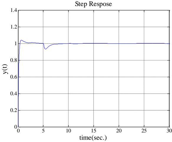
Fig. 9. Step response of the system for  $k_p = 10.1034$ ,  $k_i = 12.96$  and  $k_d = 0.3$ .
