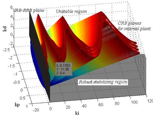
Fig. 12. Robust stability region for a *PID* controller in the  $(k_p, k_i, k_d)$  parameter space.
