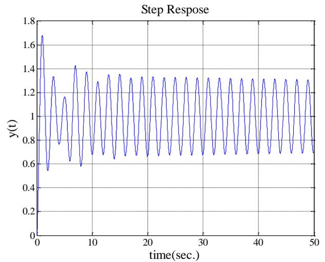
Fig. 7. Step response of the system for  $k_p = 0.1034$ ,  $k_i = 12.96$  and  $k_d = 0.3$ .
