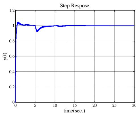
Fig. 13. Step responses of the system  $C_2(s)G_2(s)$  for 729 different values of the plant.
