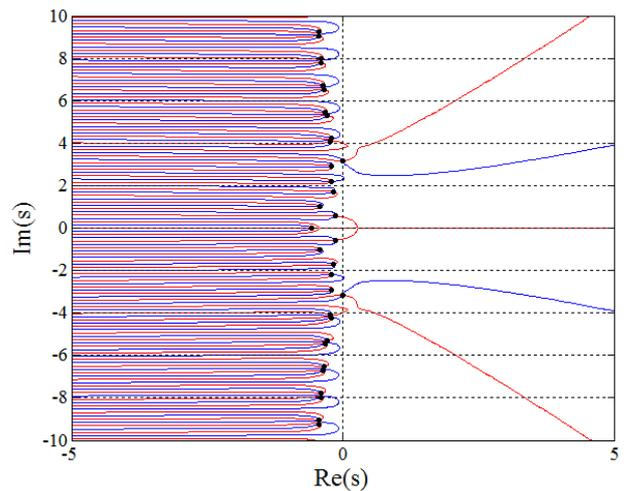
Fig. 8. The roots of the characteristic polynomial for  $k_p = 0.1034$ ,  $k_i = 12.96$  and  $k_d = 0.3$ .
