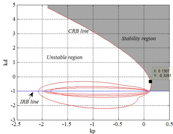
Fig. 3. Stability region in the  $(k_p, k_d)$  parameter space for the values  $k_i = 0$ .
