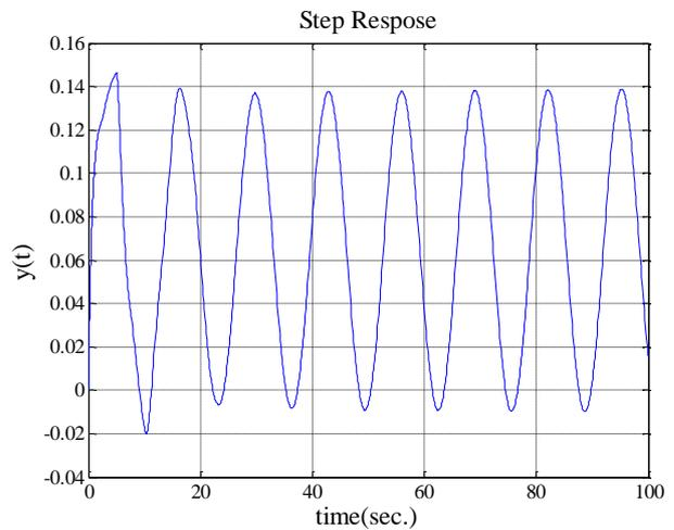
Fig. 5. Step response of the system for the values  $k_p = 0.1307$ ,  $k_i = 0$  and  $k_d = -0.3281$ .
