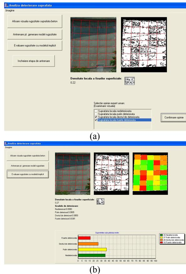
**Fig. 3.** An example sub-plot analysis and its use in: (a) the training phase, to derive fuzzy sets parameters; (b) the evaluation phase, to assess the concrete surface deterioration severity
