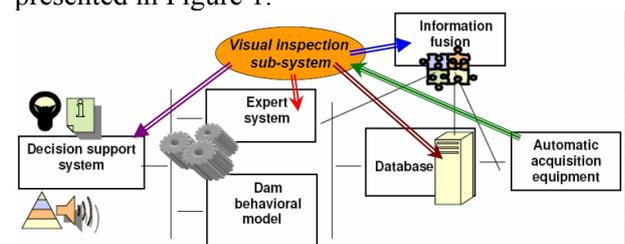
Fig.1. Integrated system for dam safety decision support
