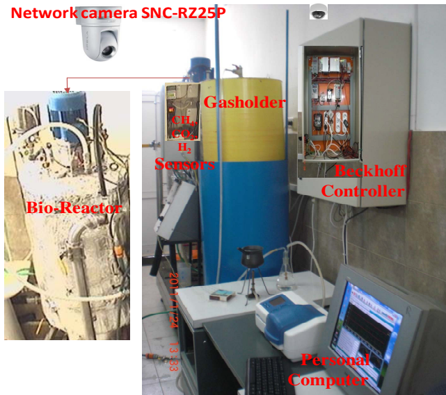
Fig. 2. General View of the real-time experimental platform
