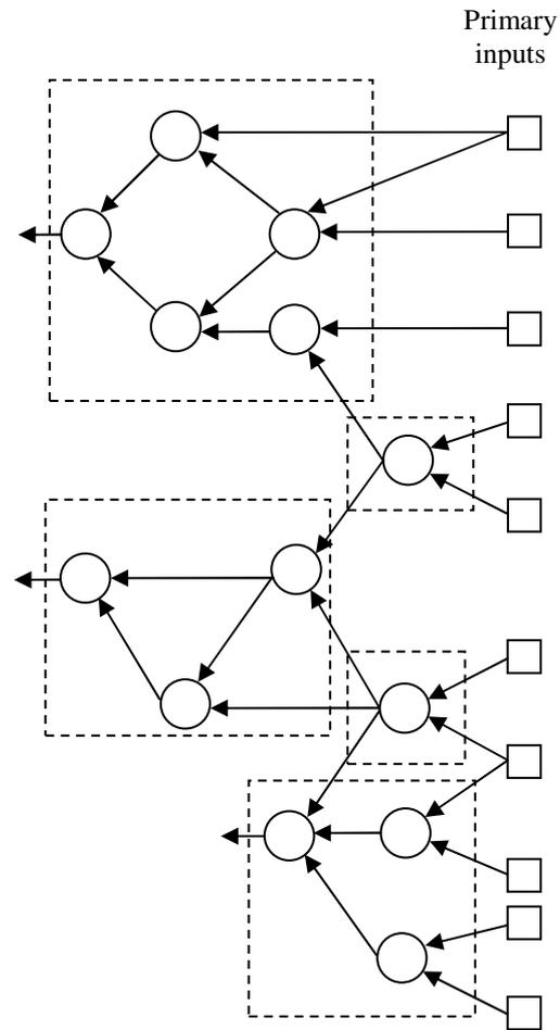
**Fig. 3.** MFFC partitioning network for duplication free mapping.
