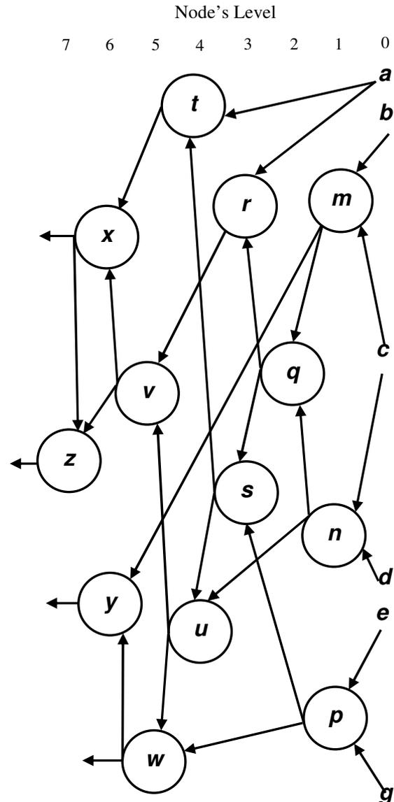
Fig. 1. Directed acyclic graph representing multilevel combinational circuit.
