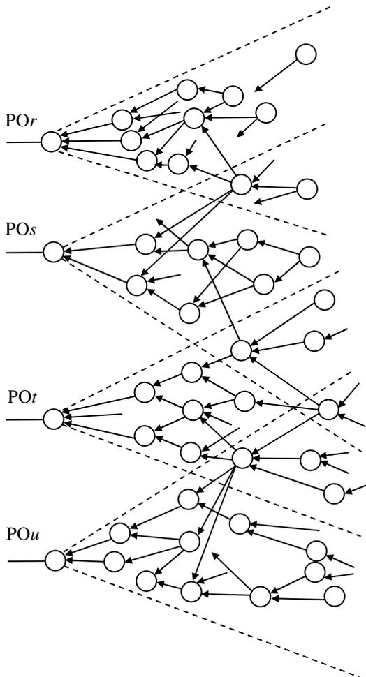
**Fig. 2.** Primary output lines and their transitive fan-in cones.
