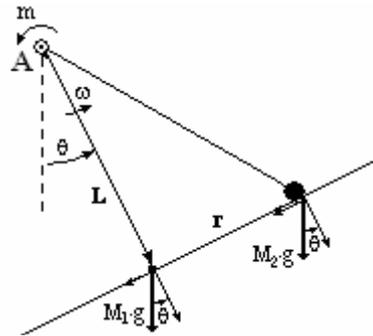
Fig.4. Ball and beam system
