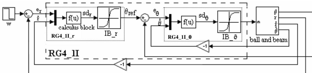
Figure 9. Interpolative based control scheme with  $RG4\_II$  for the ball and beam system.
