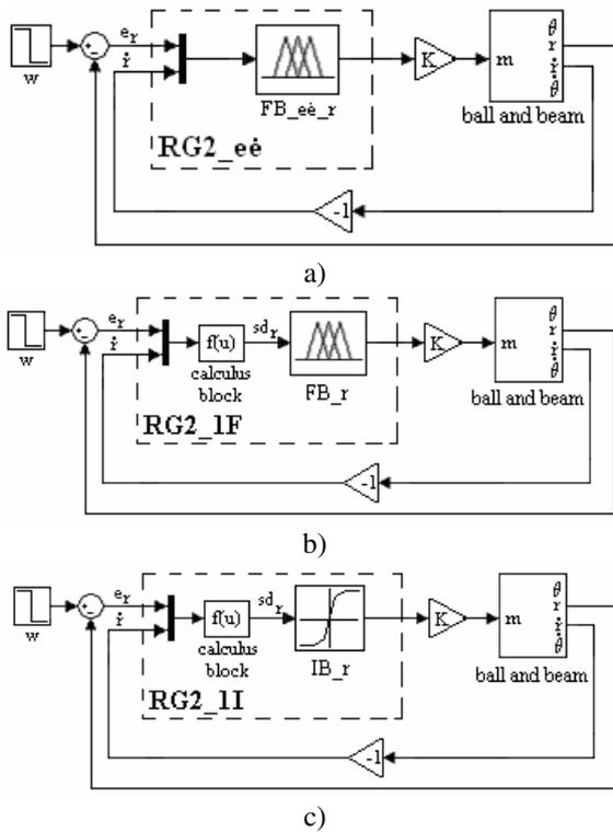
Figure 11. Fuzzy control system with  $RG2\_eè$  (a),  $RG\_1F$  (b) and  $RG2\_1I$  (c) for the ball and beam system
