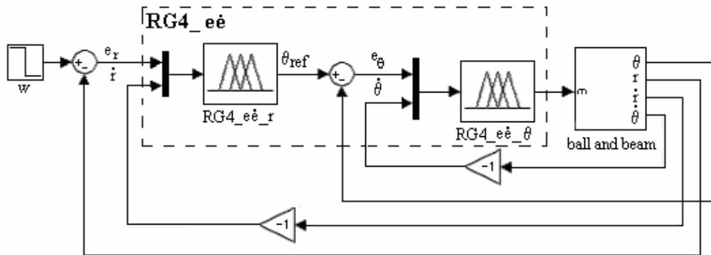
Fig.5. Fuzzy control scheme with  $RG4\_e\dot{e}$  for the ball and beam system
