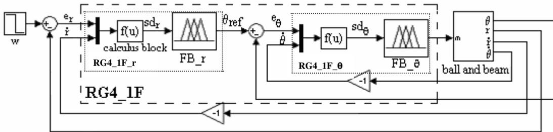
Figure 8. Simplified fuzzy control scheme with  $RG4\_IF$  for the ball and beam system.
