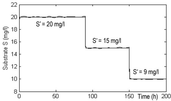
Fig. 4a. Controlled output  $S$
