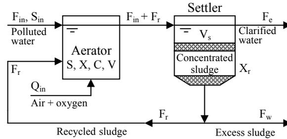
**Fig.1.** Schematic view of an activated sludge process
