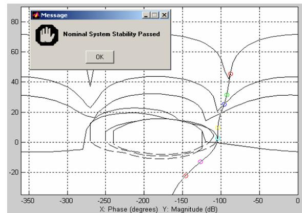
**Fig. 3.** Shaping of the open loop on the Nichols chart for the transfer function (14).
