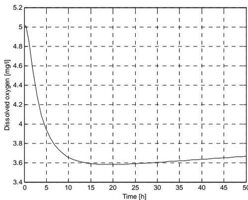
**Fig. 2.** The response of the system with PI controller designed for drought regime working in normal pluviometric regime.
