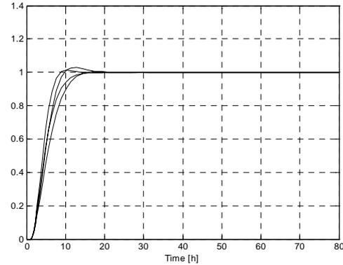
**Fig. 6.** The response of the loop using the controller (23) and the process described by different linear models for the drought regime.
