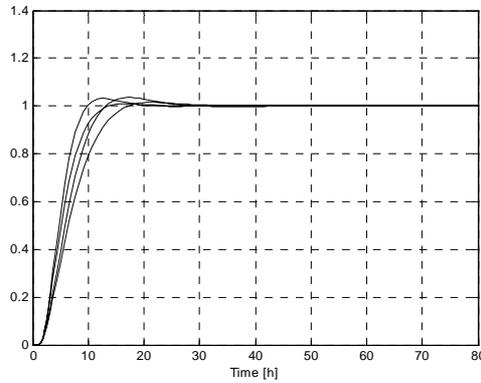
**Fig. 5.** The response of the loop using the controller (19) and the process described by different linear models for the drought regime.
