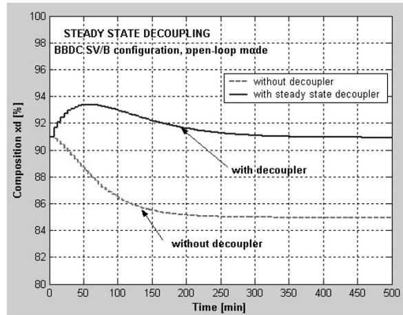
**Fig. 6.** Composition  $x_D$  to a 5% step increase of V/B, SV/B open-loop mode, steady-state decoupling.
