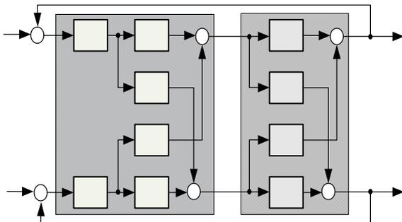
**Fig. 1.** Multivariable control system with decoupling controller.
