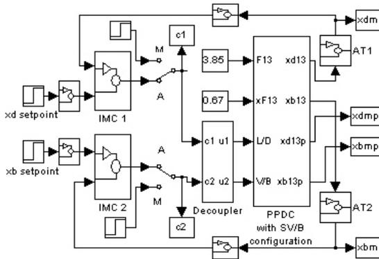
**Fig. 3.** PPDC. The Simulink model of the serial connection decoupler-distillation column.
