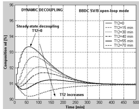
Fig. 8. Tuning decoupler time constant  $T_{12}$  to a 5% step increase of  $V/B$ .
