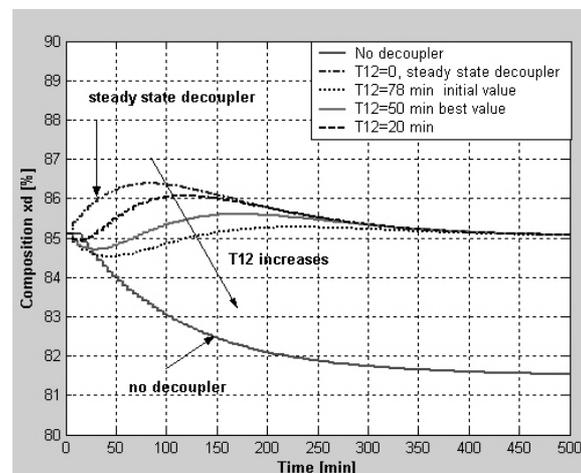
**Fig. 5.** PPDC. The composition evolution  $x_D$  to a step increase of  $V/B$  input with 5%, with and without decoupler, SV/B open-loop mode.
