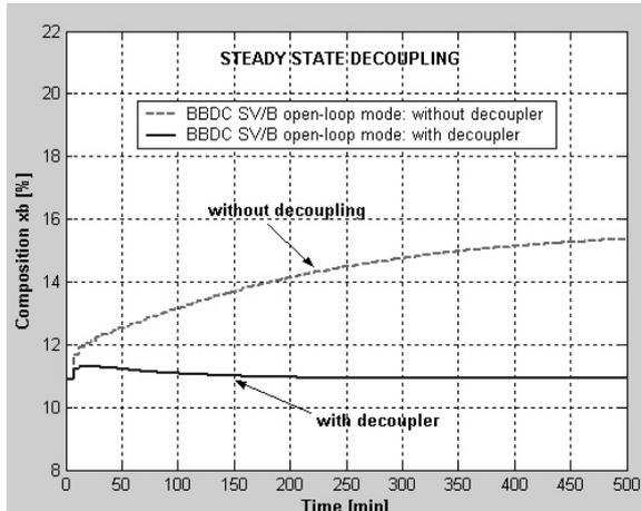
Fig. 7. Composition  $x_B$  to a 5% step increase of  $L/D$ , SV/B open-loop mode, steady-state decoupling.
