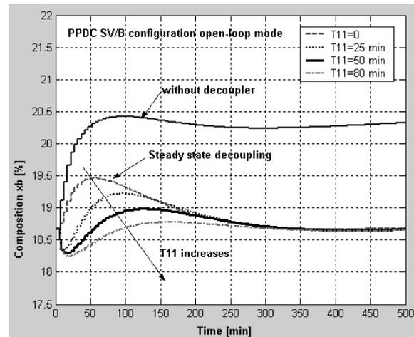
**Fig. 4.** PPDC. The composition evolution  $x_B$  to a step increase of  $L/D$  input with 5%, with and without decoupler, SV/B open-loop mode.
