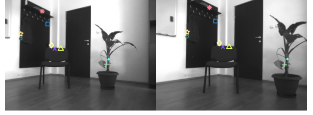
Fig. 4. Left: SURF features on the right images captured at the initial position; Right: SURF features on the right images captured after robot motion.
