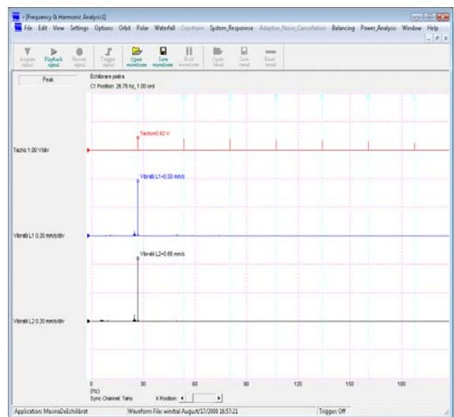
Fig. 3 The frequency spectrum of initial vibrations, in the bearings of abrasive disk.
