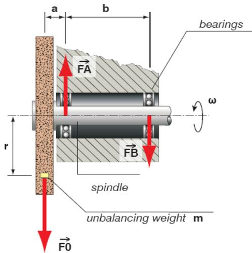
Fig. 2 Grinding wheel and its bearings.
