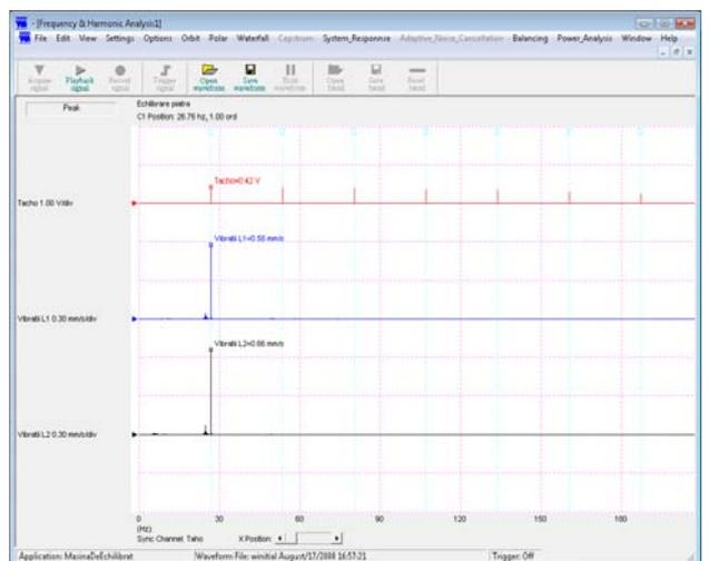
Fig. 4 The frequency spectrum of initial vibrations
